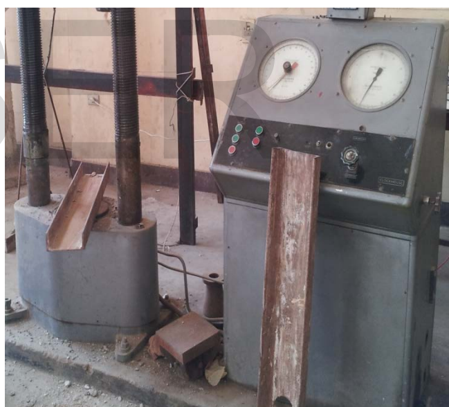
Figure (16) A steel beam as C-channel for transfer the load to wall.
