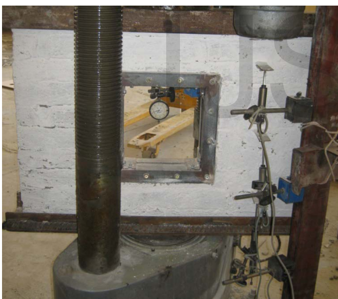
Figure (15) The used LVDT for measuring vertical strain.
