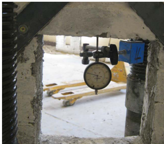
Figure (14) The used dial gauges for measuring lintel deflection.
