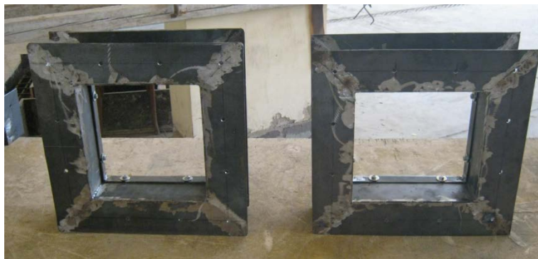
Figure (7) The used steel plate box-section.
